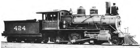
Fig. 33. Mogul (2-6-0) Two-Cylinder Compound Locomotive. Built by the Rogers Locomotive Works for the Illinois Central. Cylinders 20 in. and 29 in. x 26 in., Working Steam Pressure 200 lbs. per sq. in., Diameter of Drivers 56\frac{1}{2} in., Weight on Drivers 107,000 lbs., Total Weight 129,000 lbs.
